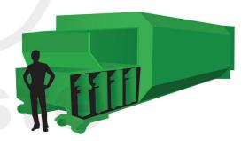
Typical open, ground loading installation. Ideal for throw-ins, truck clean-out or fork-lift use.
